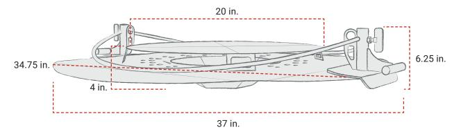
ADJUSTABLE POSITION WITH DUAL OUTPOST RODS
